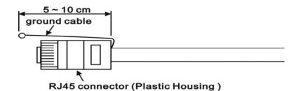
2. Make the ground cable connect to ground screw, then plug RJ45 connector.
